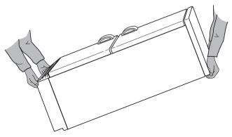
In order to push the appliance into its final position, press carefully at the top of the door and tip the appliance back slightly. The weight is thus transferred to the back casters and the appliance can be easily pushed.
